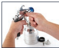
2 Slide trigger lever to release needle
