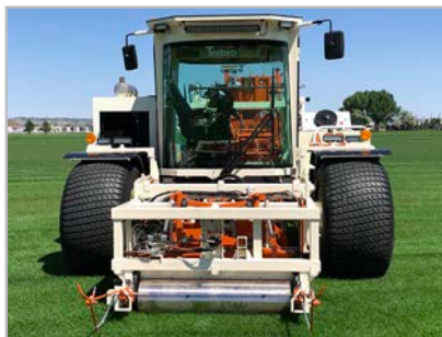
24 inch cutting heads with dual adjustable down pressure
