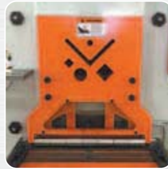
Hydraulic hold-down. (optional on IW-45K / IW-60B)
