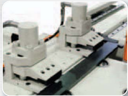
Operate in semi-automatic mode with use of gauging piece allows punching holes near the edge of the material.
