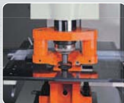
*Urethane spring stripper for minimal deformation.
