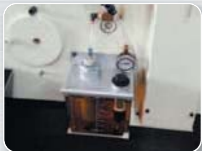
*Auto lubrication system with adjustable frequency and oil amount for longer tool life.
