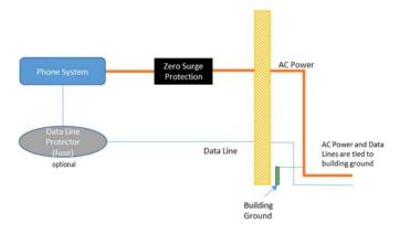
If lightning should induce a current towards your building, the copper wire is grounded at the service entrance (along with your AC power) which provides a path for the current to return to Earth without ever entering your building. If lightning strikes the building or the wires directly, nothing will protect from the extreme energy which would melt the wires.
