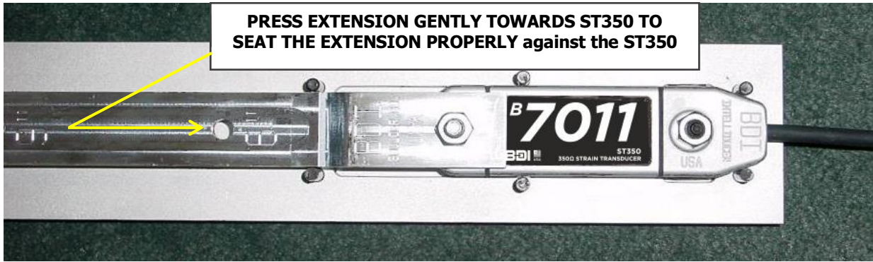
Figure 17: Aligning ST350 and Extension in the Jig
