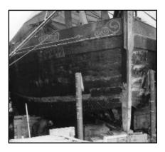
From top left to bottom right:: The rotten keel removed; the jacked up bows;new floors and frames; shipwright Baden at work on the new runs of planking in to the bottom of the barge and the chines. Photographs Pat and Peter Boss.
