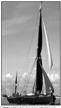
The picture on the top right shows Pudge sailing in 1996 and the drooping shape of her bows shows up by comparison with the picture at the bottom of the page taken in 2003 after the bows had been rebuilt as described in this article. However the drooping stern is also apparent in the sheer line under the vang fall in the more recent picture.
