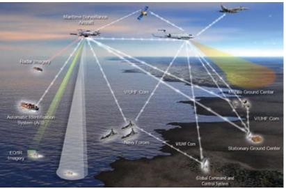
ABOVE - Schematic diagram showing how ISTAR air assets provide network connectivity. (Raytheon image)
