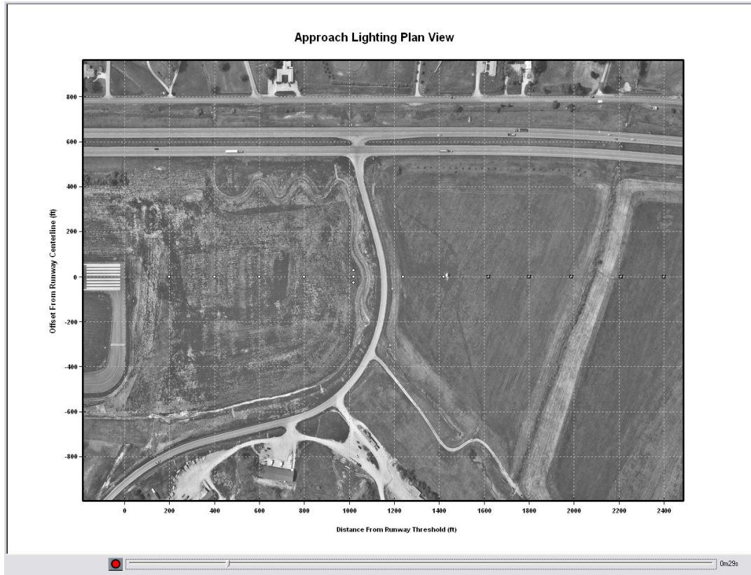
Figure 23. KUNI MALSR Output Plot Overlaying Aerial Photograph
