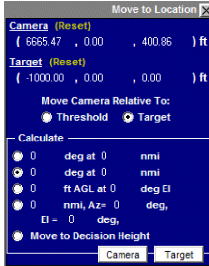
Figure 8. Window for manual entry of camera and target parameters
