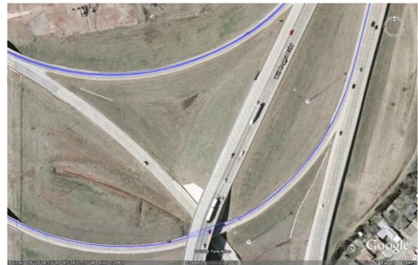
Figure 1. Geo-referenced vehicle derived ground tracks
