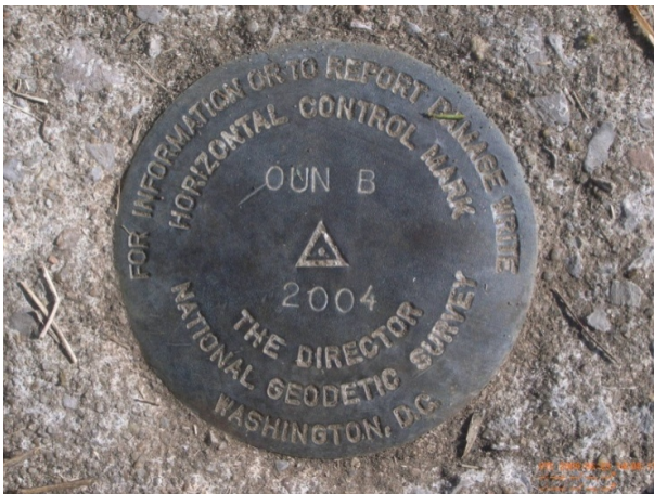
Figure 5 NGS Benchmark – Secondary Airport Control Station (SACS), Westheimer Airport, Norman, OK, USA (KOUN)
