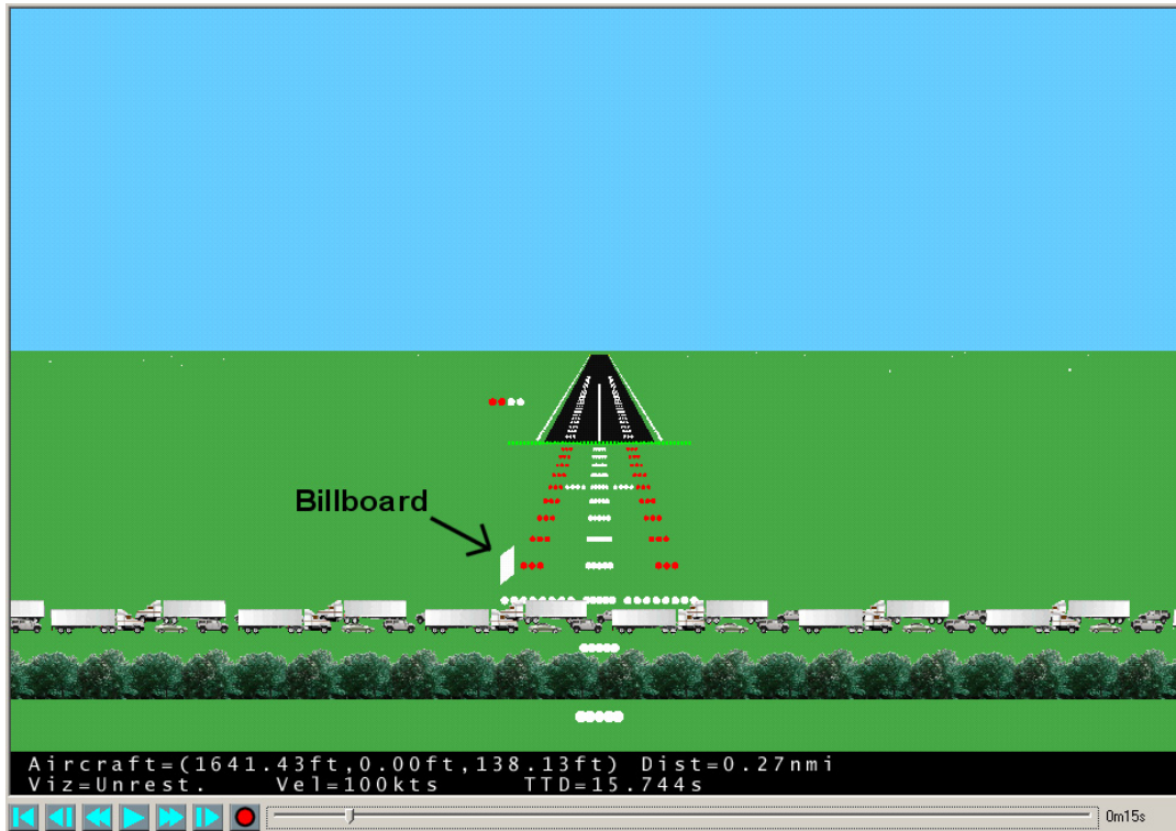
Figure 14. Pictorial showing the various object types which could potentially block the light plane.
