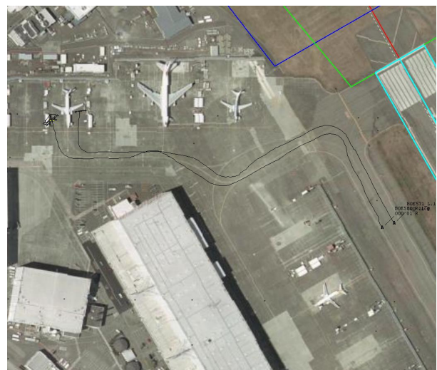
Figure 2 Taxi Operations at KBFI Using Two GNSS Mouse Receivers, Connected to the FV Toolset
