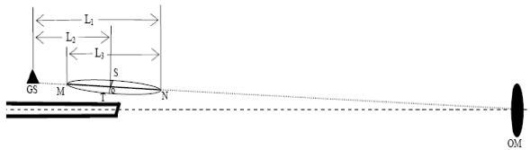
Figure 7 The Distance From Glide Slope Antenna To The Far End Of The First Fresnel
