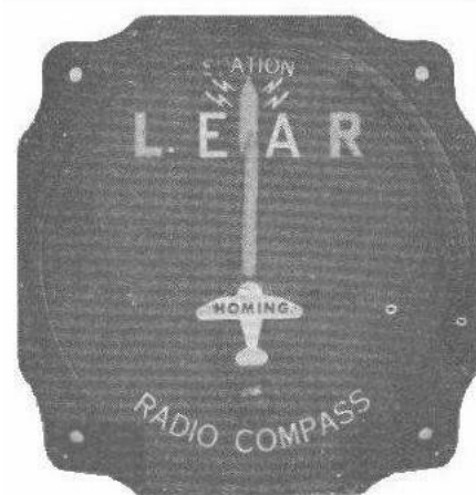
Figure 4. Lear Radio Compass (public domain)
