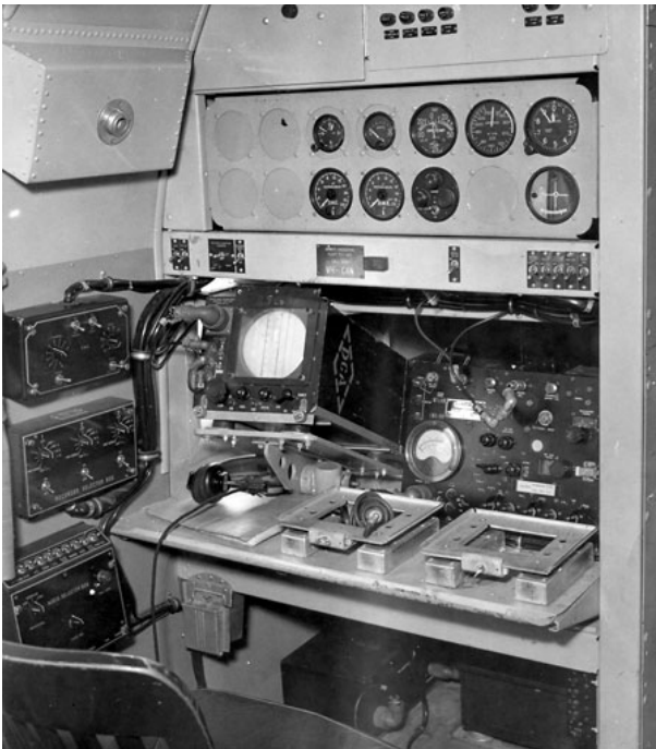
Figure 17. Circa 1954 Australia DCA flight inspection equipment, port side surveyor's station (courtesy Civil Aviation Historical Society, Inc.)
