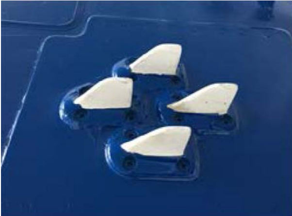
Figure 8: Cubic DF-4400 Antenna Array
