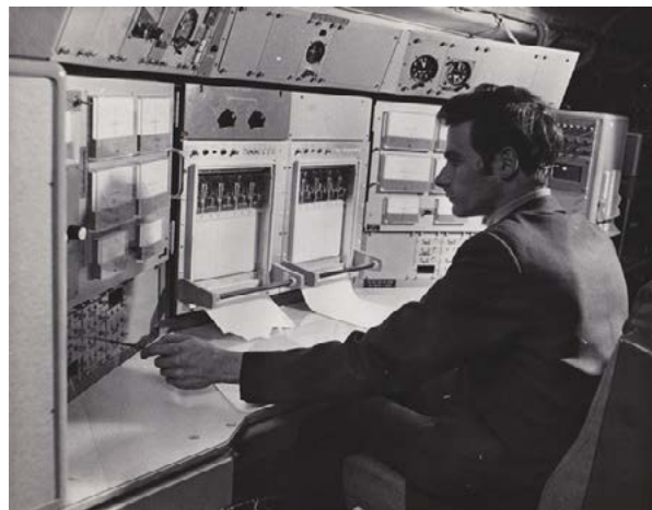
Figure 15. UK CAFU FIS installed on Avro HS-748 aircraft (from Jim Fuller collection)
