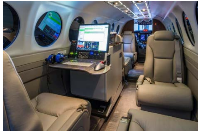
Figure 1: AeroFIS ® capable to perform ADS-B flight inspection missions
