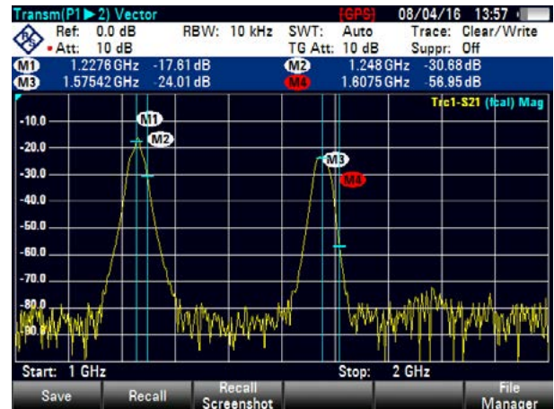
Figure 12 - Typical AFIS GPS Antenna (L1, L2)
