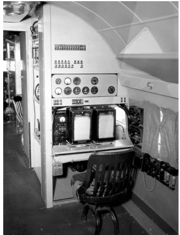
Figure 19. Circa 1954 Australia DCA flight inspection equipment, starboard side surveyor's station (courtesy Civil Aviation Historical Society, Inc.)
