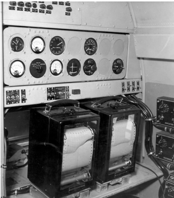
Figure 26. Circa 1954 –Australia DCA flight inspection dual equipment chart recorders (courtesy Civil Aviation Historical Society, Inc.)
