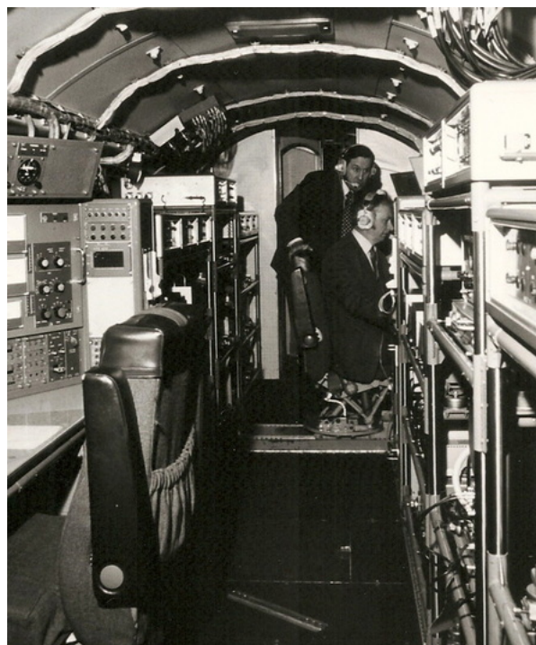
Figure 16. UK CAFU FIS installed on Avro HS-748 aircraft (from Jim Fuller collection)
