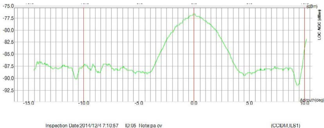
Figure 1. Signal Strength Curve of The LOC Received by Aircraft A
