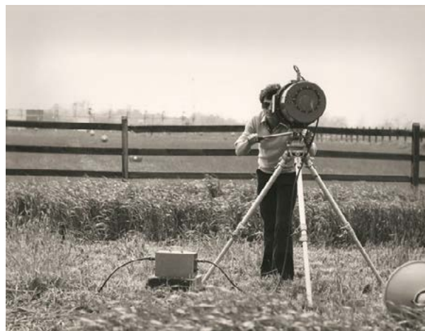
Figure 23. Infrared tracking device used for flight inspection in UK (from Jim Fuller collection)
