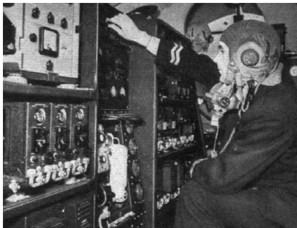
Figure 13. Circa 1952 UK CAFU flight inspection equipment installed in Dove aircraft (from Flight International magazine archives)
