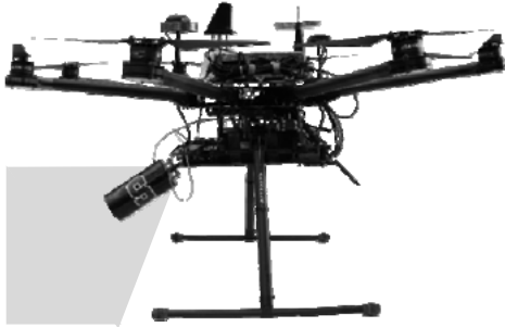
Figure 3. Directional Antenna Mounted on Underside of UAV with Antenna Main Lobe Shaded.
