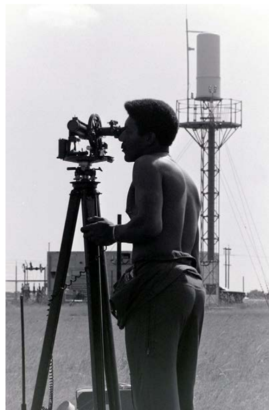
Figure 22. 1974 - USAF Theodolite operator during TACAN flight inspection at Bergstrom AFB (from USAF Flight Check Facebook Page collection)
