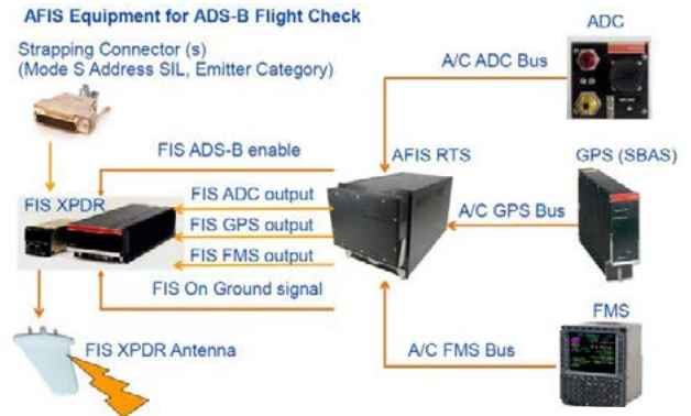
Figure 6: AFIS Configuration ADS-B Out for calibration purposes.
