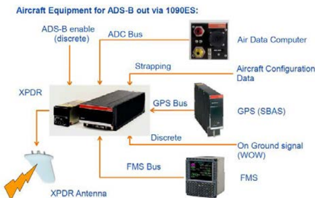
Figure 5: Aircraft Configuration ADS-B Out
