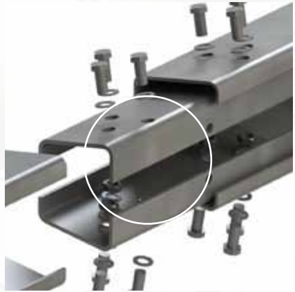
Detail showing how the Fish Plate Connectors clamp the Open Box Beam together.
