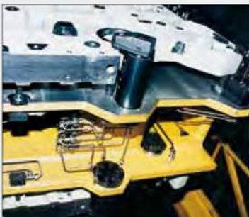
Lower flange Collet-Lok® swing cylinder mounted on a pallet.
