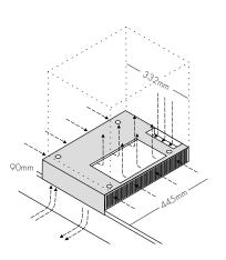
Simple-fit Ventilation Base A refined and simple-to-install ventilation kit is included with the S2 system.
