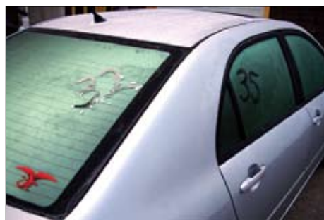
Image 2. Overall differences in window temperature detected with a 1:1 spot radiometer above. The rear window measured 0° C (32° F) while the side window appeared slightly warmer at 1.7° C (35° F).
