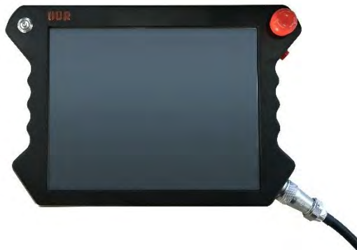
Figure 7.7 Connect straight aviation plug to teach pendant
