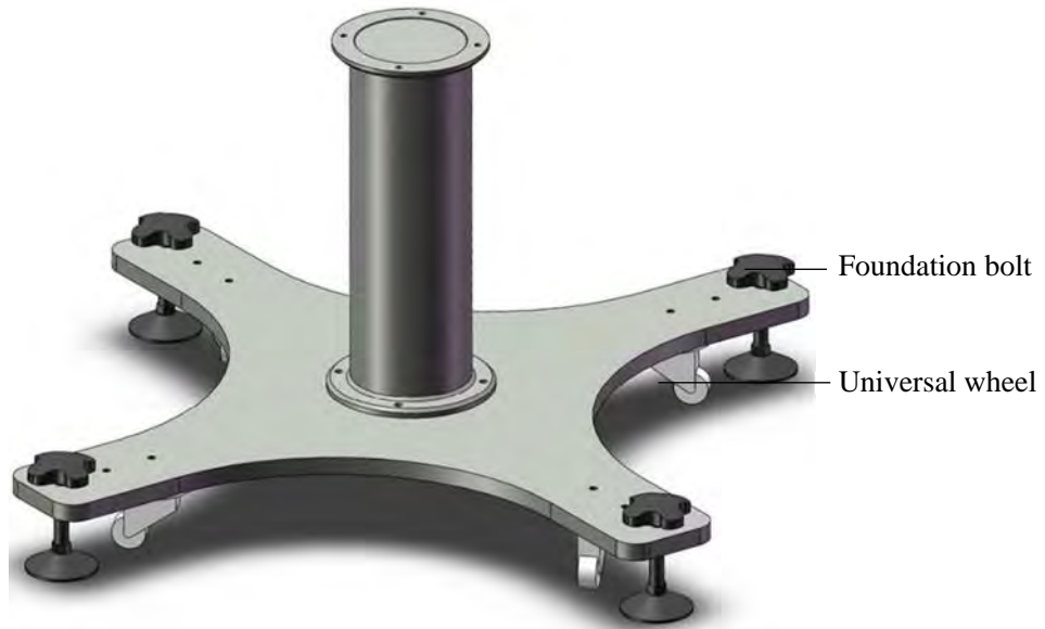
Figure 6.3 Diagram of manipulator base structure
