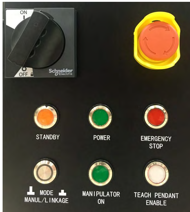
Figure 8.24 Schematic diagram of the control box front panel button
