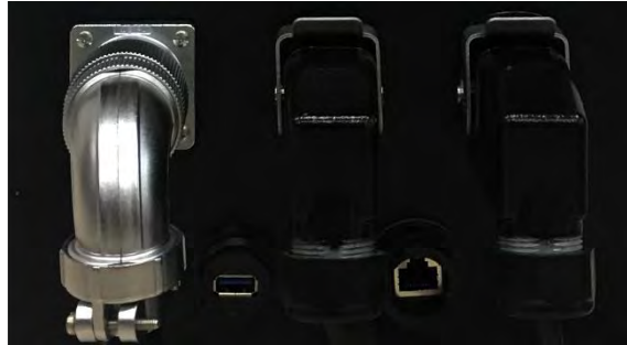
Figure 7.6 Connect aviation elbow plug cable to control box
