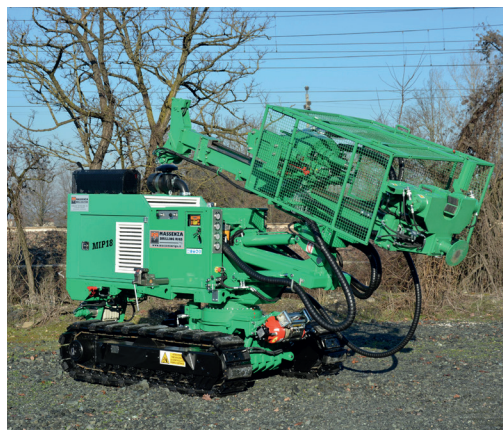
Unique Worldwide Dynamic Sampling and rotary slope climbing rig, remote control, self-levelling, drill at any angle. Photo: New for January 2017
