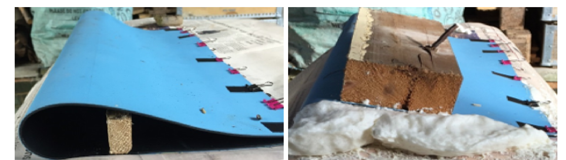
Figure 5: Manufacturing the aerofoil
