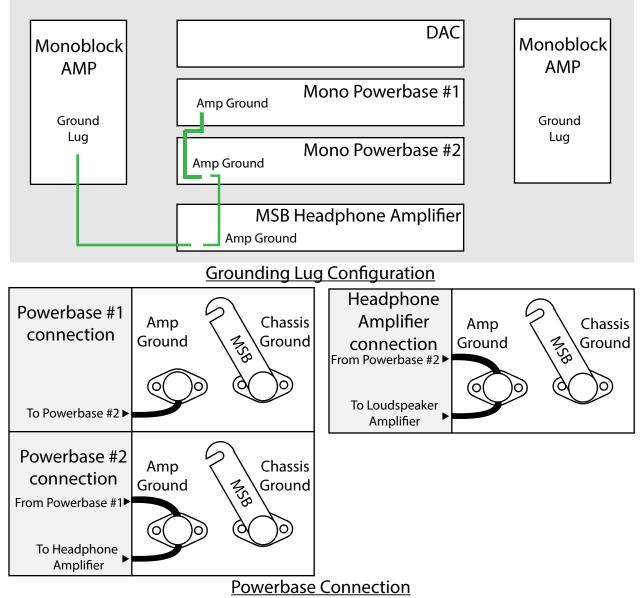
Follow the Powerbase connection method from pages 2 or 3 if using dual or mono powerbase setups. In this configuration, the Headphone Amplifier is like another powerbase in the grounding chain. After connecting your headphone amplifier continue the grounding wire to theloudspeaker amplifier in your system. If there is no ground lug on the loudspeaker amplifier, attach wire to the chassis.
