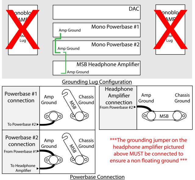
Follow the Powerbase connection method from pages 2 or 3 if using dual or mono powerbase setups. In this configuration, the Headphone Amplifier is treated as the only amplifier in the system. In this configuration, The Headphone Amplifier is the end point in the grounding chain and is much like adding another powerbase, but in this case the headphone amplifier needs to have the grounding jumper closed.
