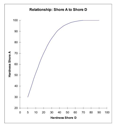
Thermoplastic Elastomers are measured in Shore A and Shore D according to ISO 868.
