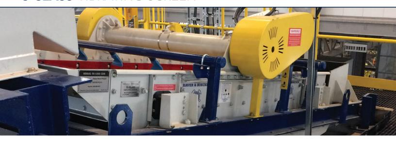
The Niagara S-Class vibrating screen is designed for fine screening slurries or dry materials within a small footprint.
