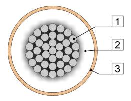
Voltage: 600/1000v Working Temperature: 250°C on the conductor Minimum bending radius: 10 x Overall cable diameter
