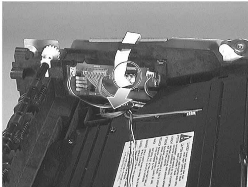
Figure 7-61 Disconnecting Power Cables
