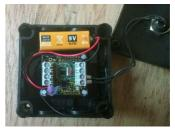
Close cover by turning each of the corner fixings % turn clockwise to align the arrow with the 'l'.
