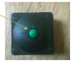
Fit the grey adapter to the post or wall within range of the gate. Check the range by operating the gate before fixing.
