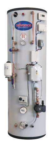
The ECB 210 is a plug and play solution for mains hot water and vented heating in the all electric apartment. The hard work is taken out of the installation as the unit is pre wired and pre plumbed. A few wiring and plumbing connections are all that is required to fit this smart stainless steel unit. It is supplied as shown.
