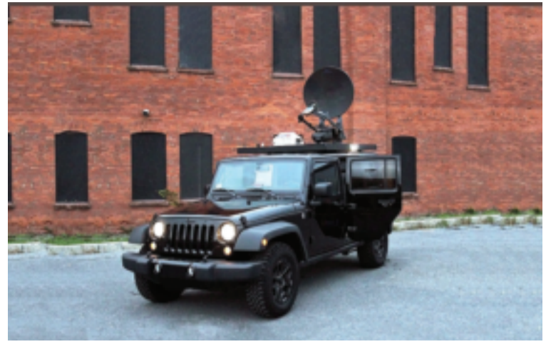
LiveU has developed an integrated satellite and cellular solution, which comprises portable and rack-mount LiveU encoders, satellite modems, and the LiveU roof-mounted Xtender with multiple cellular connections.
