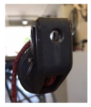
Dead ending the halyard by drilling a 5mm hole in the top of the head fitting gives an even pull and removes another potential chafe point. Use the tip of a 7mm drill to put a small countersink on the **top** and **underside** of the hole to remove the sharp edges, this is just visible in the right-hand picture above.
