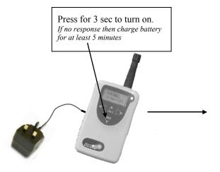
Charger can be left permanently connected or it can boost charge from empty in 8 hours
