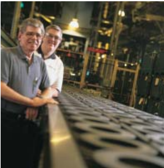
Multilane accumulation for robotic interface.
