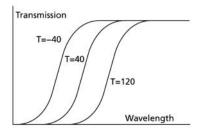
and the relationship between the specific wavelength where the absorption shift takes place and temperature is predictable.
