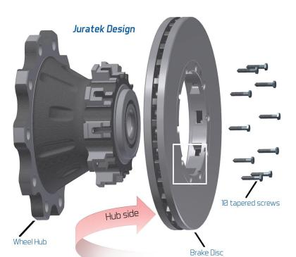
Juratek have increased the size of the intermediate splines and replaced the 10 spring washers with an integrated fixing ring.
