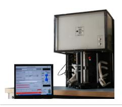
LabVIEW Real-Time module and FPGA is at the core of the MPR system. The deterministic environment is essential to MPR's precise calculations
