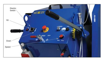
The desired cutting depth is adjusted by a motorized threaded spindle unit. In order to rise or lower the saw blade you use the electric switch on the left side of the machine panel. Turning the switch form his zero position in **two steps** to the left side and hold
