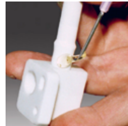
Aremco-Bond™ 526N bonds alumina to alumina ceramic.
