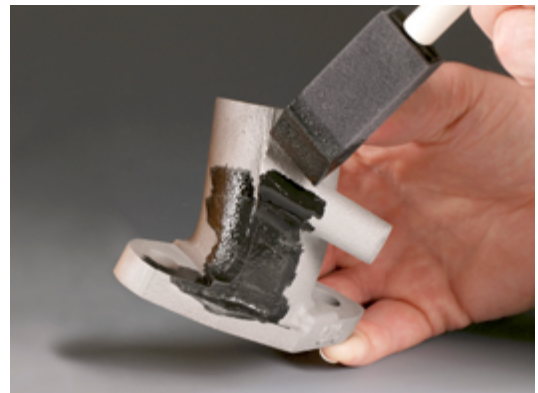
HiE-Coat™ 840-CM coats cast steel part.
