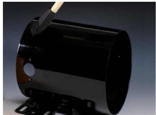
CP2000 seals thermal spray on motor housing.
