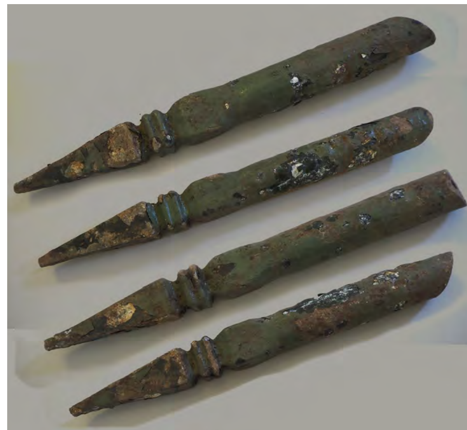
Fig. 109: Example of railing from Highgate Cemetery showing traces of original paint colours
