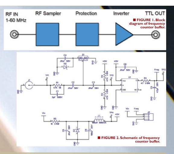
his buffer allows you to connect your counter to any RF source from 20 mW to 200 watts, from 200 kHz to 60 MHz. The circuit has a protection limiter that keeps the RF signal strength in a safe range for the TTL input of the counter, as well as providing gain for weaker signals (**Figure 1**).
