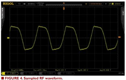
signal on 14 MHz into a 50 ohm dummy load. R1 and C1 comprise the sampling section. R1 samples some of the RF from the signal as shown in **Figure 4**. R1 has to dissipate a little of the power, so at one watt, it's somewhat bigger that you may expect. C1 shapes the frequency response and provides better sensitivity above 20 MHz as shown in **Figure 5**.
