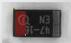
Capacitor Oriented Backwards
