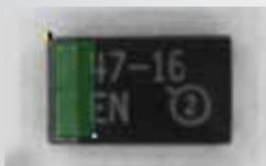
Capacitor Oriented Correctly
