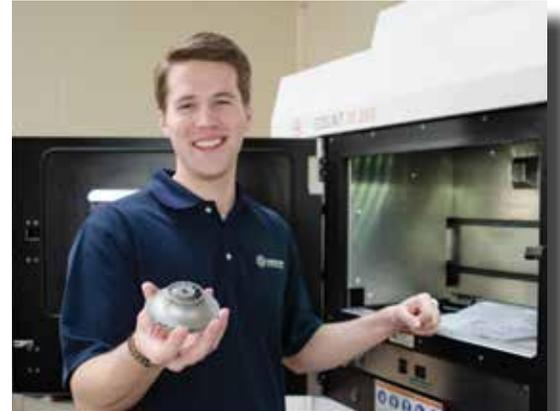
DMLS is an additive manufacturing technology that creates metal parts with highly complex geometries directly from 3-D CAD data in hours instead of days or weeks and without any tooling. The software “slices” the model into thin layers which the DMLS machine then builds layer by layer, fusing metal powder into a solid part by melting it locally using a focused laser beam.
