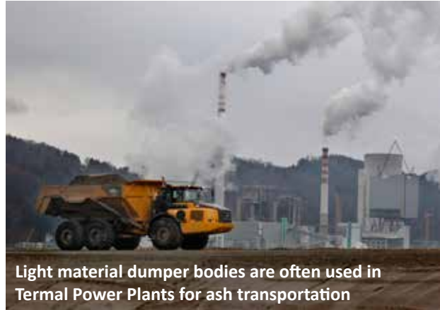
Dumper body can be firmly closed (sealed) so it is also appropriate for liquide materials transportation
