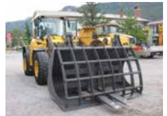
Bucket with clamp made on Balavto Ltd. for loader Volvo L70
