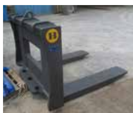
Forks for stone blocks made for loader Michigan L270, Capacity 60 t
