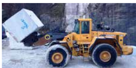
Forks for stone blocks made for loader Michigan L270, Capacity 60 t
