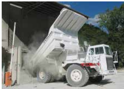
Model DP 405 WD Weight (empty): 29,8 t Capacity: 40 t Power SAE J1995: 410 kW (550 HP) at 2100 rpm
