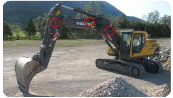
'View Line' system on the excavator
