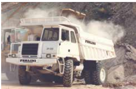
Model DP 255 Weight (empty): 17,8 t Capacity: 30 t Power SAE J1995: 298 kW (400 HP) at 2100 rpm
