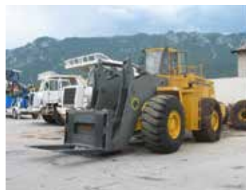
Forks for stone blocks made for loader Michigan L270, Capacity 60 t
