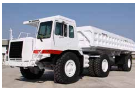
Model DPT 70 (combination between rigid and articulated dumper) Weight (empty): 45 t Capacity: 70 t Power SAE J1995: 410 kW (550 HP) at 2100 rpm
