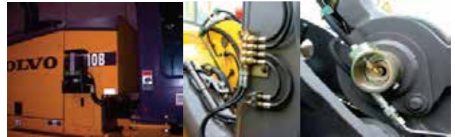
Automatic greasing system mounted to the machine
