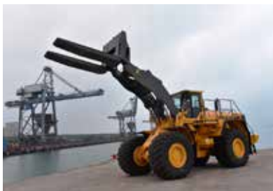
Forks for stone blocks made for loader Volvo L350F, Capacity 80 t
