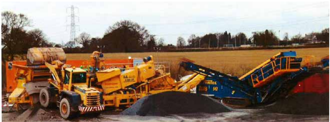
Whole complex: Bruce screener for sand washing, system for water recycling and slime draining
