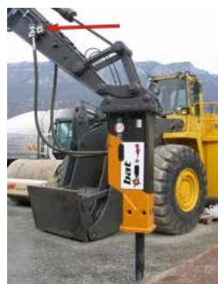
Hydraulic Breaker and Shear connected to excavator with B-Quick coupler
