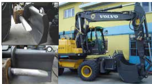
Hydraulic Breaker Carrier - an excellent help during a hydraulic breaker transportation from one site to another.
