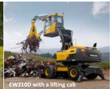
Model EW210D with regular and a lifting cab.
