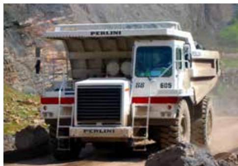
Model DP 605 Weight (empty): 38,9 t Capacity: 53 t Power SAE J1995: 567 kW (760 HP) at 2100 rpm
