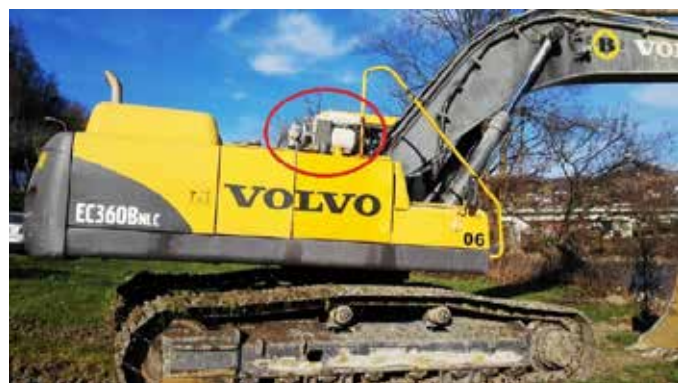
Hydraulic compressor mounted to the excavator
