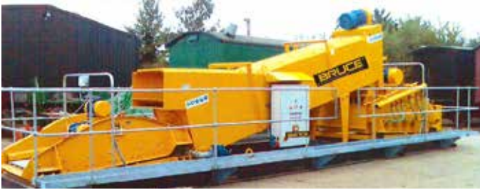
Bruce systems for washing sand and other aggregates
