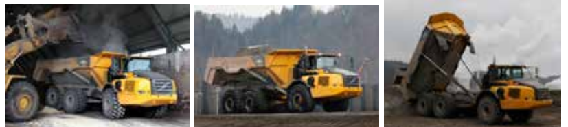
Dumper body can be firmly closed (sealed) so it is also appropriate for liquide materials transportation
