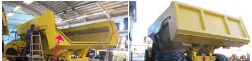
Dumper body can be firmly closed (sealed) so it is also appropriate for liquide materials transportation
