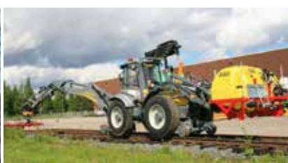
The Lännen Rail multifunction machine - equipped with everything necessary for work on and around railway tracks
