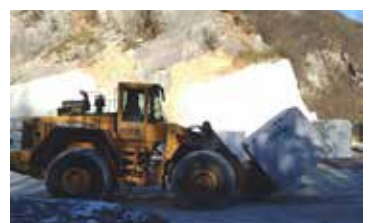
Forks for stone blocks made for loader Volvo L220, Capacity 48 t
