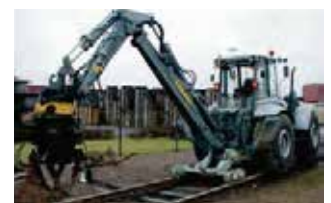
Tiltrotator for unlimited attachment rotation and tilting up to 40° in two directions
