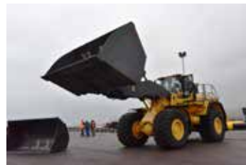
Bucket for light materials made on Balavto Ltd. for loader Volvo L350F
