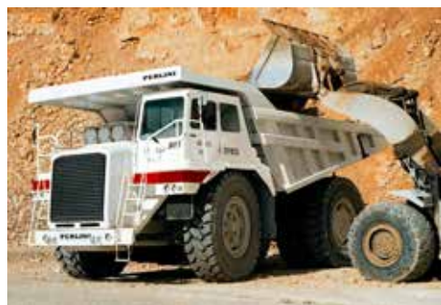
Model DP 905 WD Weight (empty): 64 t Capaity: 95 t Power SAE J1995: 783 kW (1050 HP) at 2100 rpm
