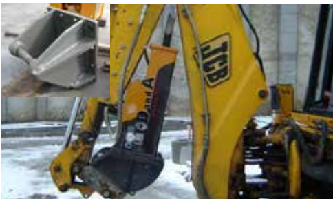
Special attaching plate for hydraulic breaker on backhoe loader.
