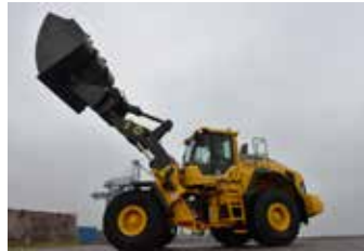
High tip bucket made on Balavto Ltd. for loader Volvo L180H
