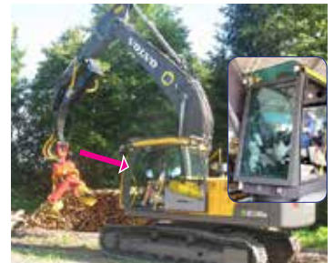
Special Protective Cab Glass on excavator cab.
