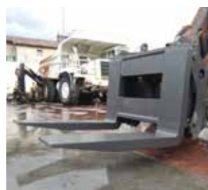
Forks for stone blocks made for loader Volvo L220, Capacity 48 t
