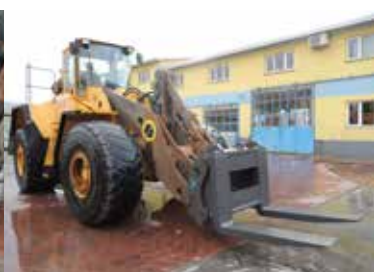
Forks for stone blocks made for loader Volvo L220, Capacity 48 t
