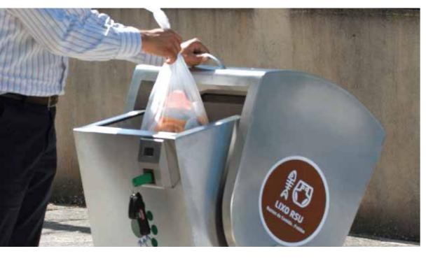
The access control module SOTKIS is a solution to apply the implementation of the waste variable rate system based in Pay-As-You-Throw (PAYT).
