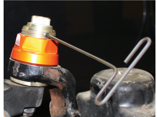
Remove the red caps, and install the load carrying cap by hand.
