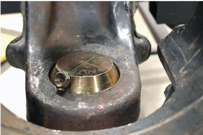
Install flush mount grease fitting in the lower ball joint.
