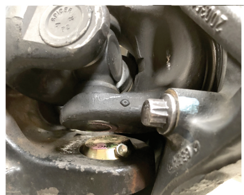
Install axle shaft and wheel hub. Ensure the axle shaft does not hit the lower ball joint grease fitting. To do this, rotate the axle shaft while turning the knuckle lock to lock.
