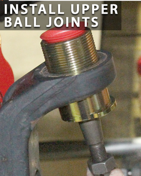
Install upper ball joint. Rare Parts design presses in from the bottom of the inner "C".
