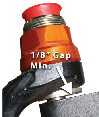
Install dust boot for the lower ball joint. Install knuckle and thread on lower ball joint castle nut. Reinstall speed sensor bracket (JK only) and thread on upper castle nut. Be sure there is a minimum of 1/8" gap between upper ball joint face and face of the knuckle.
