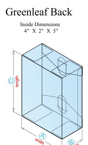
Greenleaf closures are used almost exclusively in plastic carton structures and will stand up to substantial abuse without disengaging. Greenleaf Back cartons must be hand erected, filled and closed. The locks on the back of the carton keep the front, top and bottom panels clear for graphic treatment.
