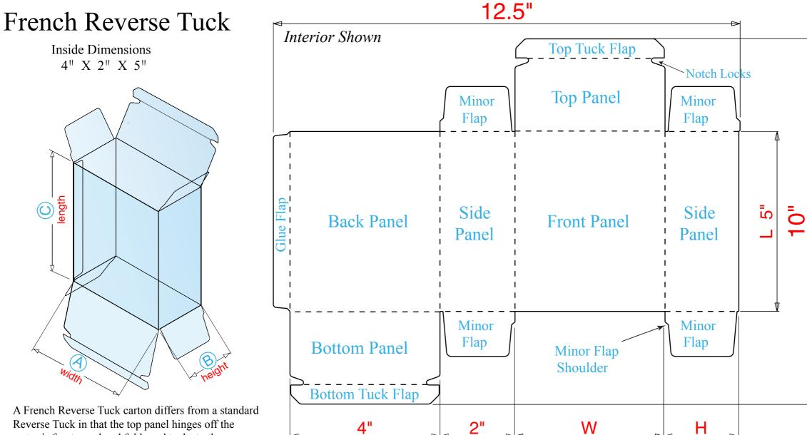
Reverse Tuck in that the top panel hinges off the carton's front panel and folds and tucks to the rear, while the bottom panel hinges off the back panel and folds and tucks to the front.
