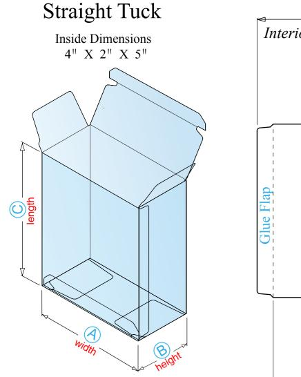
Straight Tuck cartons have both top and bottom panels that hinge off the carton's front panel. The top and bottom panels fold from the front and tuck to the rear, providing a clean front panel appearance. This style carton is appropriate for both hand and machine forming and filling applications.
