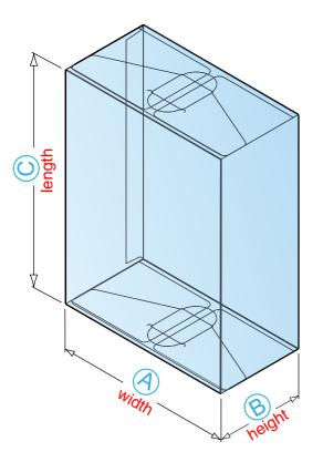
Greenleaf closures are used almost exclusively in plastic carton structures and will stand up to substantial abuse without disengaging. A Greenleaf Top & Bottom carton must be hand erected, filled and closed.
