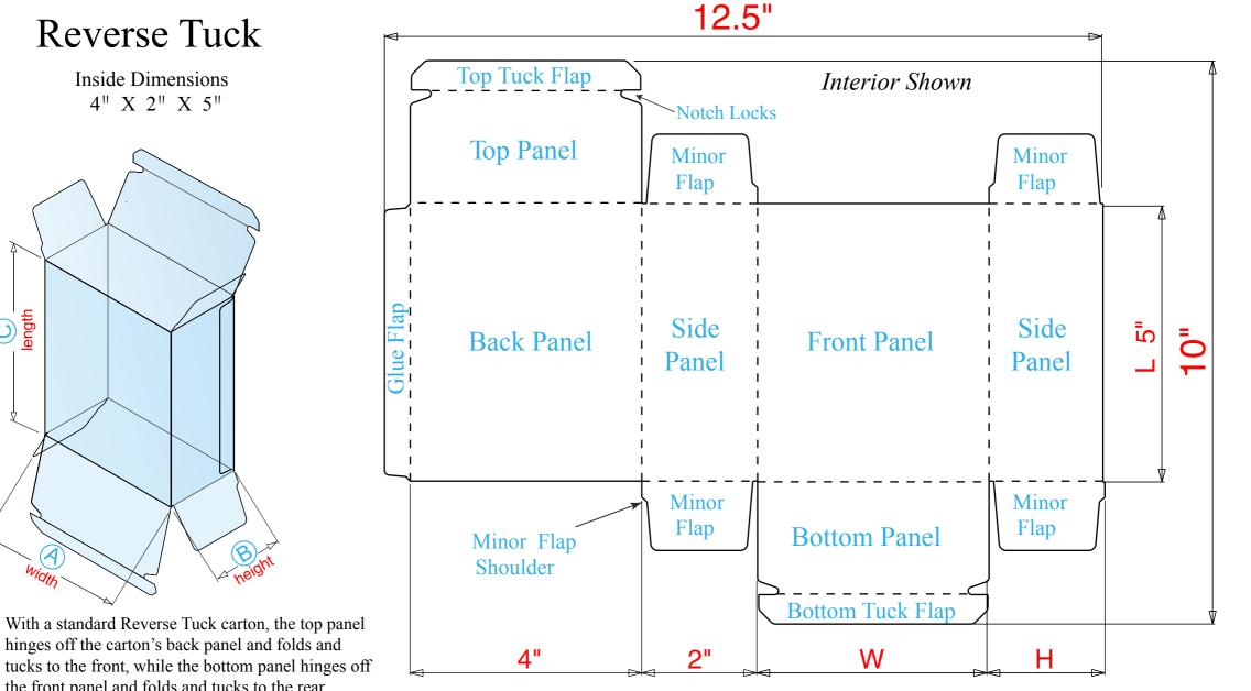
tucks to the front, while the bottom panel hinges off the front panel and folds and tucks to the rear. This style carton is appropriate for both hand and machine forming and filling applications.
