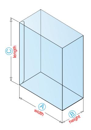
A Sleeve is used in combination with another packaging component. It's frequently used as a slip-on cover for a paperboard carton or tray, or an open set box structure. Sleeves can also be used in combination with injection molded or vacuum-formed plastic end caps or inserts.
