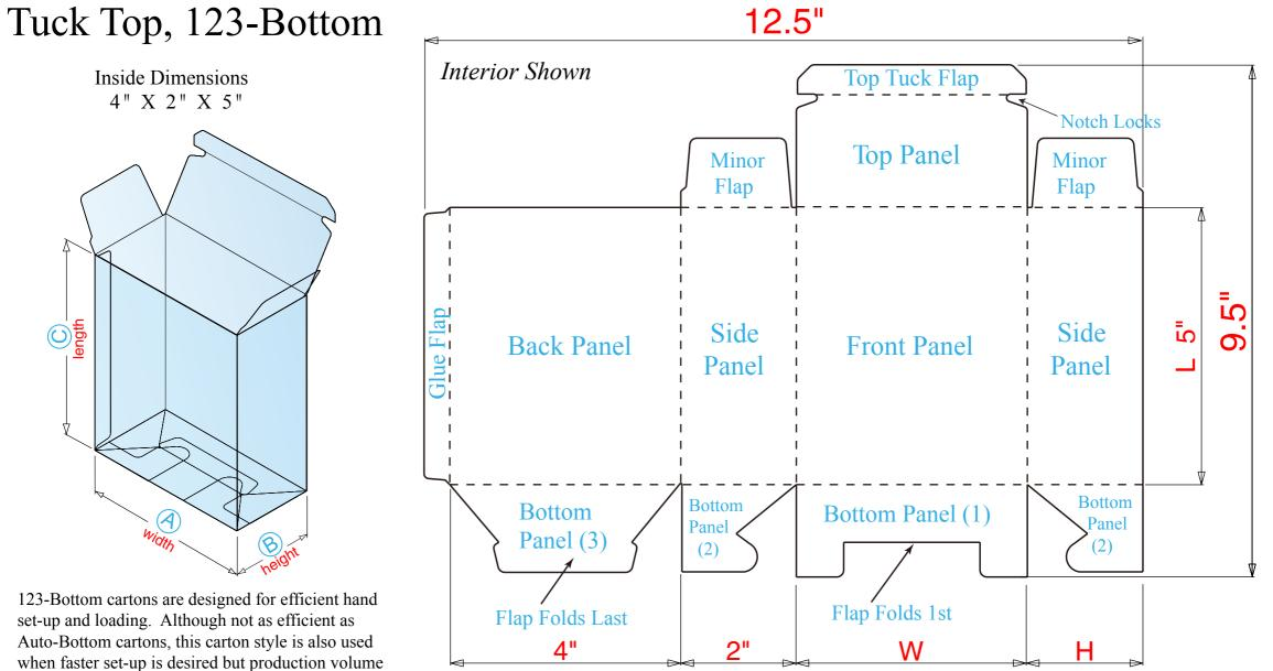
when faster set-up is desired but production volume or the package's contents are not suitable for automatic packaging equipment.
