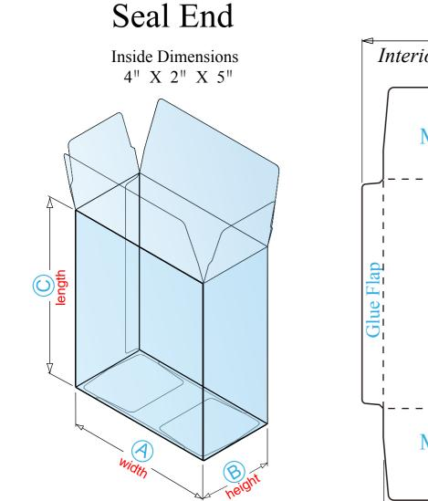
The Seal End carton is typically erected, filled and sealed on automated packaging equipment. Since the top and bottoms are glued closed, it offers tamper evidence as compared to tuck style cartons.
