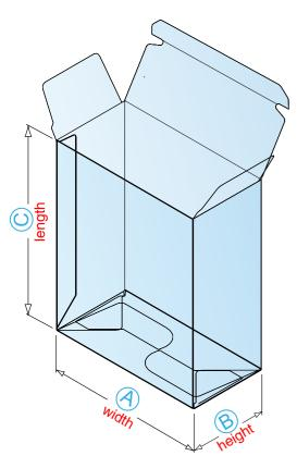
Auto-Bottom cartons are designed for efficient hand set-up and loading, and are generally used when faster set up is desired but production volume or the package's contents are not suitable for automated filling equipment. Bottom panels are pre-glued during the carton's manufacturing process.
