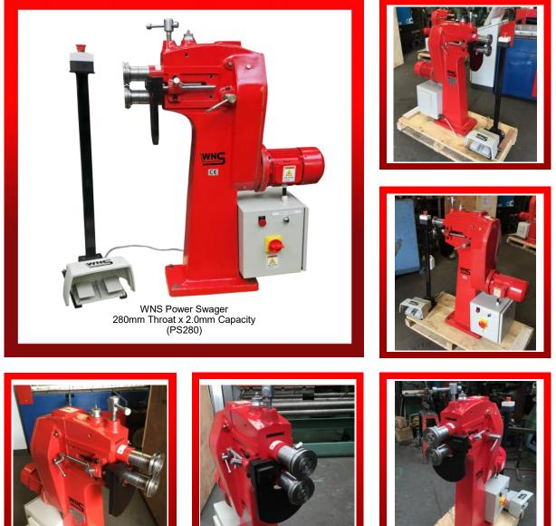
**WNS** POWER SWAGERS (PS280) are principally used for Swaging, Beading, Wiring, Crimping and Forming of sheet metal. The Power Swager has a 280mm Throat and can accommodate mild steel sheet up to 2.0mm thick. This machine comes complete with 1 Set of 3/8" Swage Rolls. The PS280 has a variable speed and a low voltage Forward & Reverse foot pedal.
