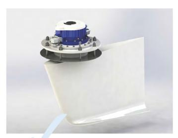
SR SYSTEM—SHORT RANGE - Starting from the experience with Stabilis Electra, the system is aimed at boats of less than 20 m. In particular it has a latest generation innovative Brushless Torque electric motor, there are three different sizes available) linked to a reducer. With its unique design, this new system ensures maximum compactness, increasingly low-wage, low energy consumption and even simpler installation. It can also be powered with 24V DC.
