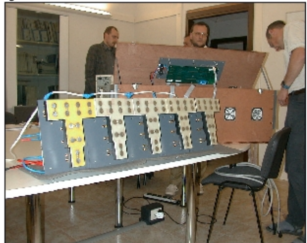
Fig. 3 - Underside of the polarimetric antenna array with its all five modules in the foreground. The radar demonstrator packaging is in the background.
