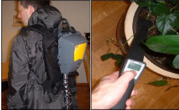
Fig. 4 - Main unit of the Biosensor sample collection system which may be carried in a similar manner to a backpack and the use of a sampling probe.
