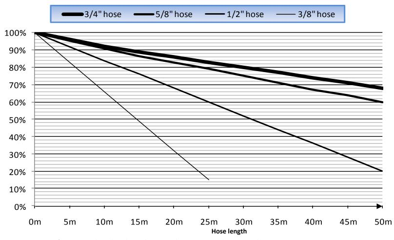
Pressure from power pack: 150 bar., Flow: 30 l.p.m., zero elevation, 2 set couplings per 10 m hose.
