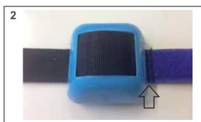
Pull the IceQube in place. The blue velcro starts right after the housing of the IceQube, as indicated by the arrow above.
