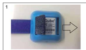
Push the straight end of the strap into the housing of the lceQube as shown and feed through the other side. Note that the blue velcro is facing outwards.
