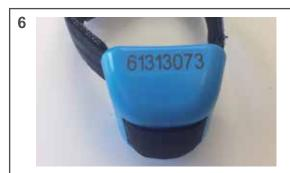
The unique indentification number on the housing of the IceQube should still be facing up.
