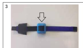
Make sure the IceQube as shown here is positioned such that the unique identification number on the housing faces up.
