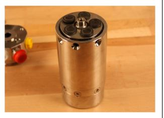
11. Mount the new O-ring on the swash plate and lubricate with clean filtered soap water. Place the swash plate on top of the pistons. Turn the pump upside down and place it on the tool for mounting the bearing while holding on to the swash plate. Make sure to orient the swash plate threads towards the holes in the house. Be careful not to squeeze the O-ring. Press down until it slides into place. Mount the 5 screws while pressing downwards.
