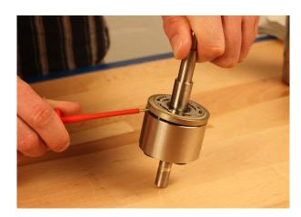
5. Remove the 5 screws holding the house attached to the port flange.
