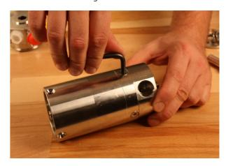
10. Mount the spring, retainer guide, retainer plate and pistons. Please confer with the exploded view at the end of this instruction for correct orientation.
