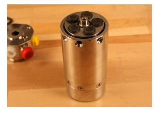
3. Continue pressing the shaft into the pump to get the cylinder barrel out
