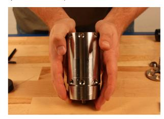
Mount the 5 screws. Lubricate the screw thread with grease. Tighten with firm torque. Make sure not to over-tighten the screws.
