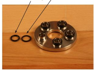
6. Wet the liners and O-rings/back-up rings with clean filtered soap water. Place the valve plate on top of the cylinder barrel and press gently downwards.
