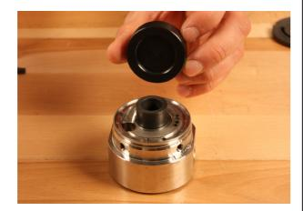
4. Mount the pin and the port plate. Replace the O-ring, if required.
