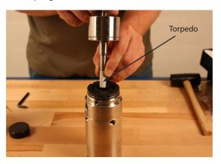
8. Lubricate the O-ring on the port flange with clean filtered soap water. Place the house on top of the port flange. Make sure to orient the port flange towards the holes in the house. Be careful not to squeeze the O-ring. Press down until it slides into place. Do not press on the shaft, as the cylinder barrel will be pressed out.
