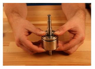
7. Lubricate the shaft with filtered soap water. Mount the cylinder barrel in the port flange. Use the torpedo in order not to damage the shaft seal by the sharp edge on the shaft.
