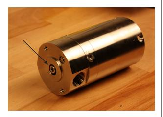
Gently lever the valve plate assembly free with the aid of a screw-driver
