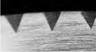
MICROSCOPIC VIEW OF A CVD INFILTRATED DRESSING DISCS EDGE
