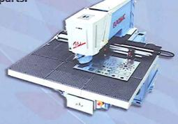
Euromac High Speed Programmable, Punching System with Multiple Tool Capability.
