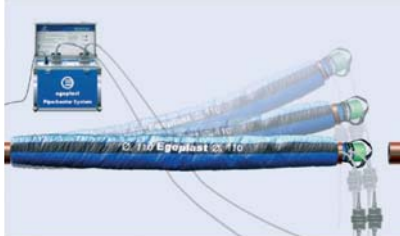
Fig 8-14: Straightening bundled coil and drum ends with the egeplast pipe-heater system
