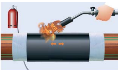
Fig 8-43: Attaching the heat shield and applying the heat shrink product
