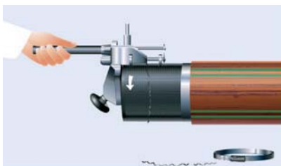
Fig 8-20: Removal of the oxide layer using a rotary scraper
