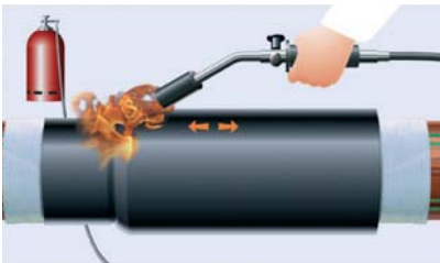
Fig 8-28: Attaching the heat shield and applying the heat shrink product
