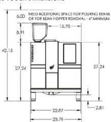
NEED 4" MINIMUM SPACE BEHIND UNIT AND WALL FOR PROPER AIR CIRCULATION
